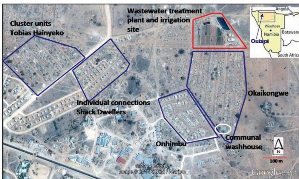
Figure 1. (Color online) Map of the planned sanitation, wastewater treatment and agricultural reuse facility in Outapi. Blue: connected settlements, red: wastewater treatment plant, irrigation fields, storage pond, evaporation pond, white: communal washhouse (satellite image is provided with permission by CNES/Astrium 2013, powered by Google Earth. Map of Namibia: Röhrig 2011, adapted).
